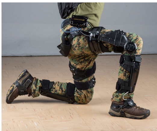
The exoskeleton Onyx, developed by Lockheed Martin Company, which improves the soldier's endurance and capacities. © 2021 Lockheed Martin Corporation
